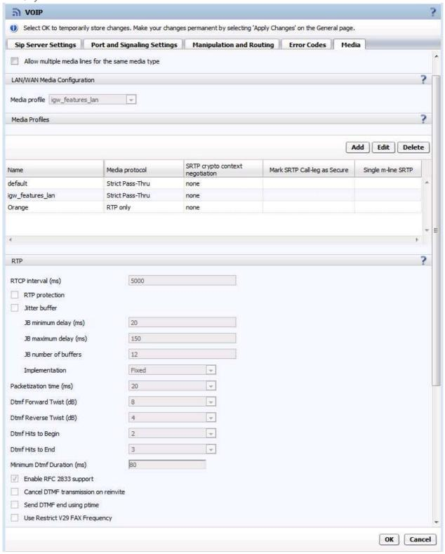
In the used Media Profile *Orange* must be configured the settings below to meet Orange requirements.
