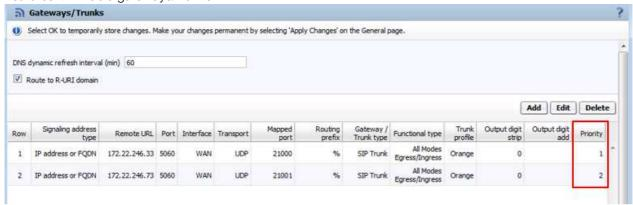
In this configuration the nominal Orange SBC 172.22.246.33 has priority 1 and the seconds Orange SBC 172.22.246.73 has priority 2.
