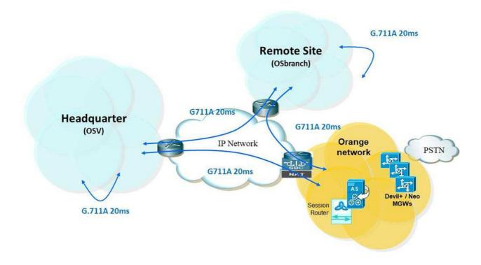
Call routing on OS Branch is as follows. The phone is registered via OS Branch with OS Voice so the phone is registered with both servers.
