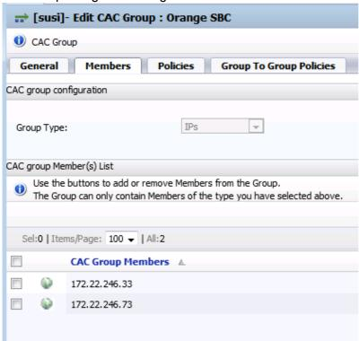
Here are configured the IP addresses of both Orange SBC's as Group Type IPs.
