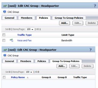
Adding or opening the **Traffic Type** entry on the Policies tab the **Limit Type** and **Max Bandwidth** can be configured:
