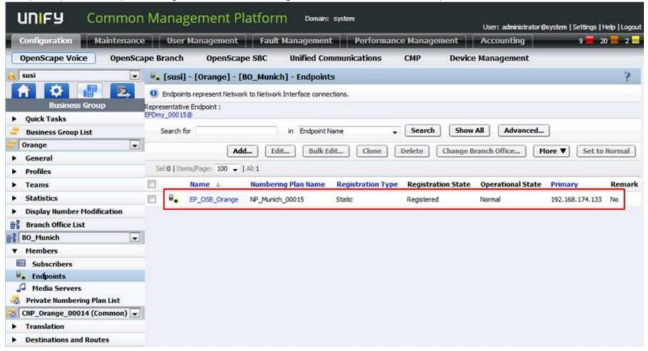
Below is shown the configuration of the OpenScape Branch endpoint for the virtual LAN IP:
