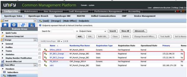
The backup SBC is used in case the nominal SBC does not respond within the time specified in the Outgoing Call Supervision Timer, see below.
