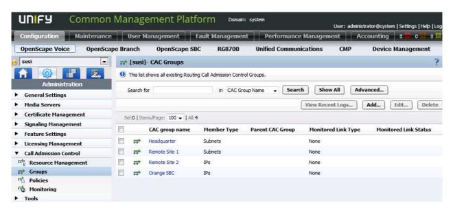
For each CAC Group is configured codec restriction to **G.711 A-law** and **Voice and Fax** as Traffic Type. If no restriction of bandwidth is required in a CAC Group its value should be set to the highest value possible.
