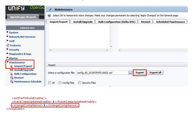
In case the exported configuration file does not show the *orangeCompliance* flag the auto refresh timer on GUI must be changed and applied by clicking on Apply Changes, and afterwards the export must be done again.
