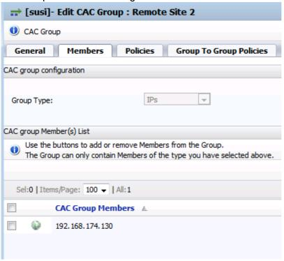
Here is configured the OpenScape Branch IP address as Group Type IPs.
