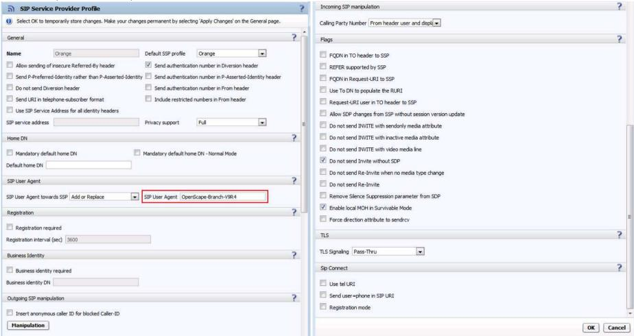
In the SIP User Agent towards SSP field must be configured the OS Branch version as string to meet an Orange requirement.
