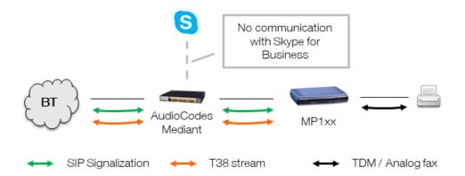
In this architecture fax device is connected to AudioCodes MediaPack 1xx analog telephony adapter. MediaPack is integrated with Mediant which can be placed in other remote site or in datacenter. Mediant gateway with no directly connected endpoints can be virtualized.
