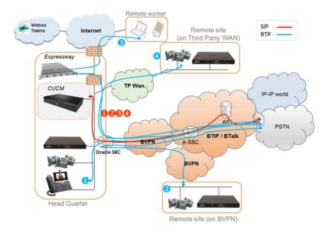
In this architecture, all SIP trunks are anchored by the Oracle Enterprise SBC. The call flows are very similar to the architecture with Cisco CUBE. Session Border Controller is mostly transparent for SIP traffic. It can also be used for TLS encryption ensuring secure traffic between Oracle ESBC and Orange SBC.
