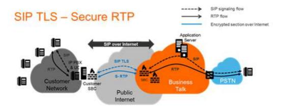
In this architecture, all SIP trunks are anchored by the CUBE in flow-through mode for the media. Traffic between CUBE and Orange A-SBC is carried over public internet. The traffic is encrypted with TLS v.1.2 for signalization and SRTP for media. CUBE on ISR G3 chassis performs transcoding between RTP and SRTP by default therefore internal traffic within customer site can be unencrypted.
