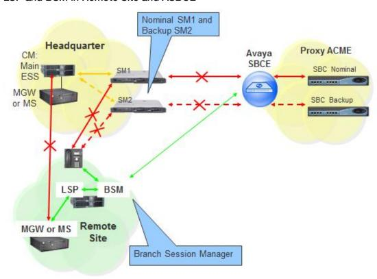
When communication from Remote Site to the Primary Controller (main ACM server) and Survivable Core Server (ESS) is lost then the Remote Site's IP telephones and Media Gateways and Media Servers register to the Survivable Remote Server (LSP) and SIP telephones register to the Branch Session Manager.
