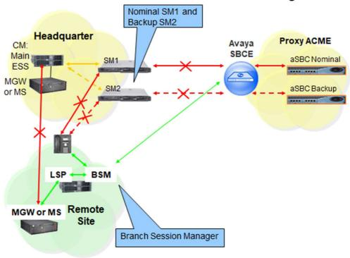
When communication from Remote Site to the Primary Controller (main ACM server) and Survivable Core Server (ESS) is lost then the Remote Site's IP telephones and Media Gateways and Media Servers register to the Survivable Remote Server (LSP) and SIP telephones register to the Branch Session Manager (BSM).
