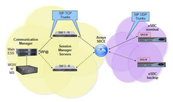
When the Survivable Core Server (ESS) is implemented in the architecture and the communication to the Primary Controller (main ACM server) is lost then all the IP telephones and Media Gateways and Media Servers register to a Survivable Core Server (ESS).
