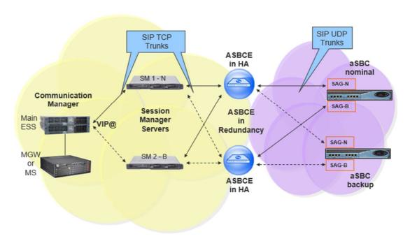
ASBCE in Redundancy mode deployment (Geographic-redundant deployment) is a multiple ASBCE deployment. ASBCE in redundancy can be deployed in the HA (High Availability) or non-HA mode. ASBCEs in redundancy are available at the same time and the calls can be routed over them depending on the dialplan on ACM/SM or AS (Application Server).
