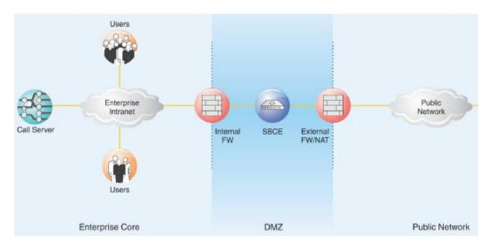
Avaya SBCE is positioned at the edge of the network in the DMZ. Avaya SBCE is directly inline with the call servers, and protects the enterprise network against all inadvertent and malicious intrusions and attacks.
